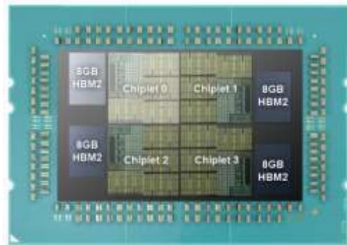
Manticore: 4096-core chiplet-based prototype architecture
