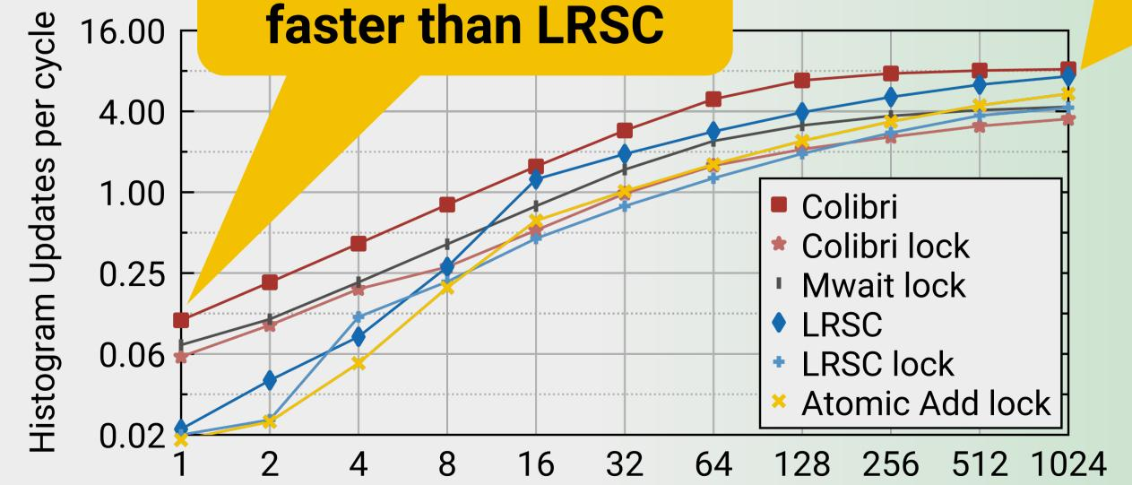
Evaluate the throughput of different atomic readmodify-write operations and lock implementations at varying levels of contention.
