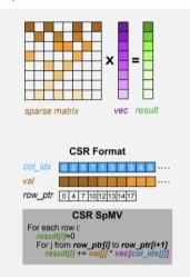
Handle indirect accesses near memory Stream indirect elements from main memory Smart Memory Controllers<sup>[1]</sup>
