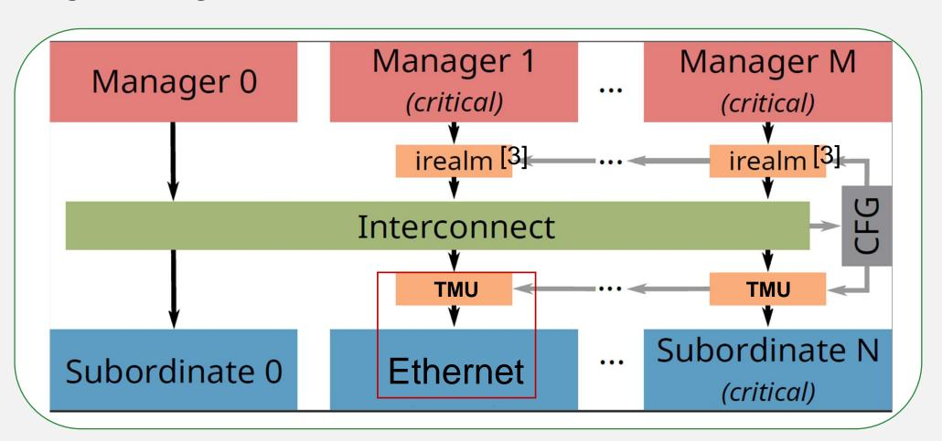
We synthesized TMU in GF12 technology under four configurations: FC and TC, with and without prescaler.
