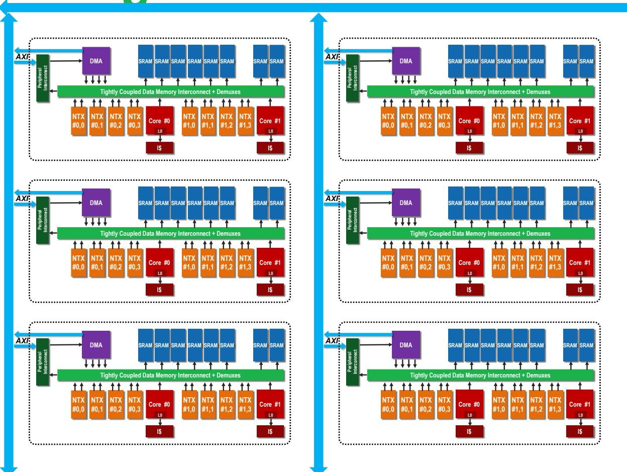
Many clusters are connected through a higher level interconnect (e.g. AXI) to scale up computing performance
