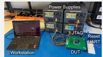
We set up a 2D (frequency, voltage) sweep, sequencing 832 sessions to create an enhanced Schmoo<sup>5</sup> plot:
