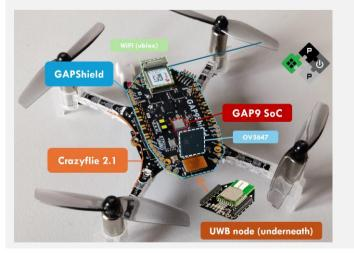
GAP9Shield[3] integrating the GAP9 SoC with 10 RISC-V cores. The shield and the UWB Loco Positioning Deck [4] are mounted on the Craziflie 2.1 nano-drone [5].
